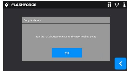
(5-5) Wait for the extruder verifying distance between nozzle and plate on the first point. If the distance on the first point is appropriate, tap[OK] to move to the next point to do the leveling. If the distance on the first point is not appropriate, operate according to the instruction on the touch screen, then tap [Verify] again.
