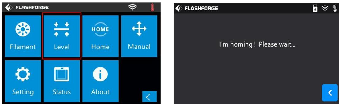
(5-1) Tap [Level] to start leveling. Wait while the extruder and platform finish homing movements.
