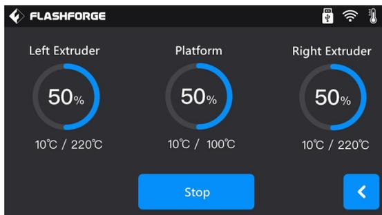
Tap the **[Preheat]** button to enter the preheat interface. Tap the **[Start]** button to heat up to the target temperature.
