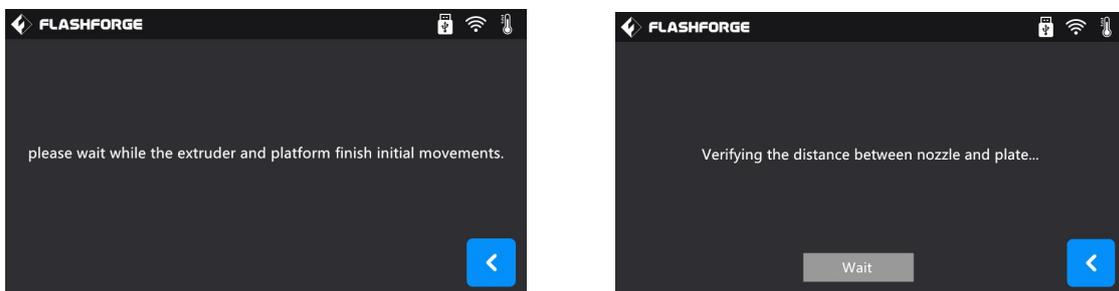
(5-3) Wait while the extruder and platform finish initial movements, Extruder move to the first point to do the leveling. Wait for the extruder verifying distance between nozzle and plate.
